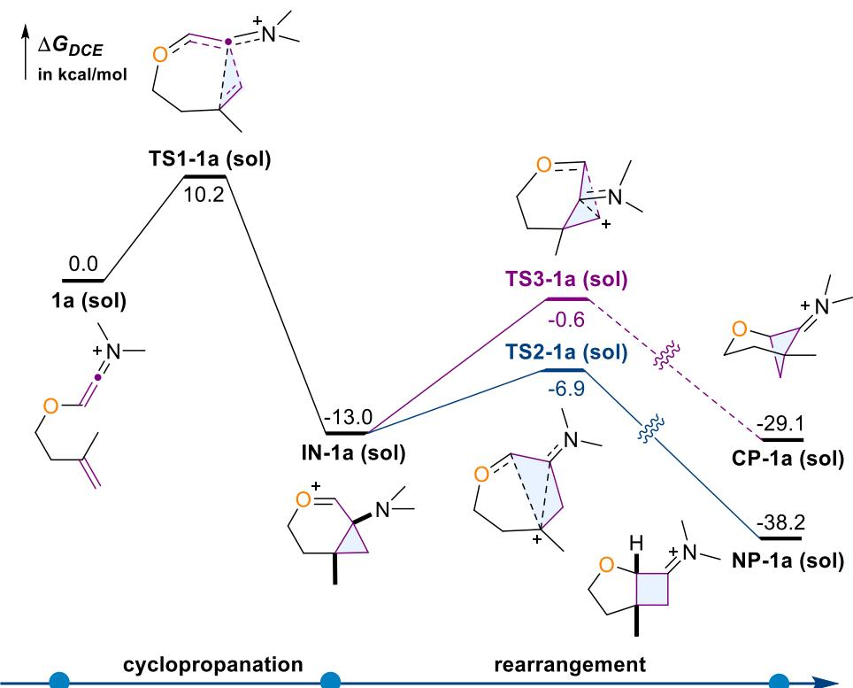
Figure S23. Gibbs energy profile based on solution phase geometry optimization for [2 + 2] cycloaddition of **1a**. Computed at DLPNO-CCSD(T)/cc-pVTZ: SMD(DCE)//SMD(DCE)/ $\omega$ B97X-D/def2-SVP level.
