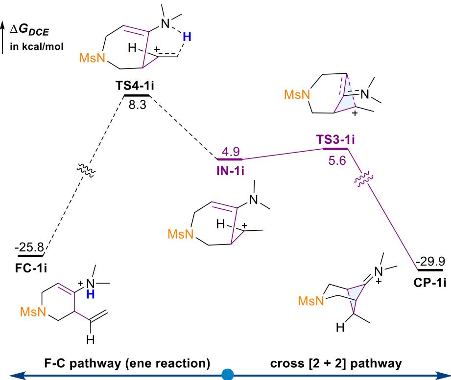
Figure S11. Comparison of F-C pathway and cross [2 + 2] pathway of **IN-1i**. Computed at DLPNO-CCSD(T)/cc-pVTZ:SMD(DCE)// $\omega$ B97X-D/def2-SVP level.
