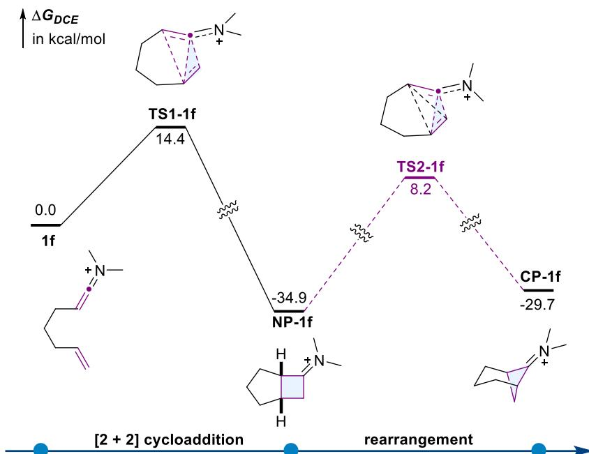
Figure S14. Gibbs energy profile for [2 + 2] cycloaddition of **1f**. Computed at DLPNO-CCSD(T)/cc-pVTZ:SMD(DCE)// $\omega$ B97X-D/def2-SVP level.
