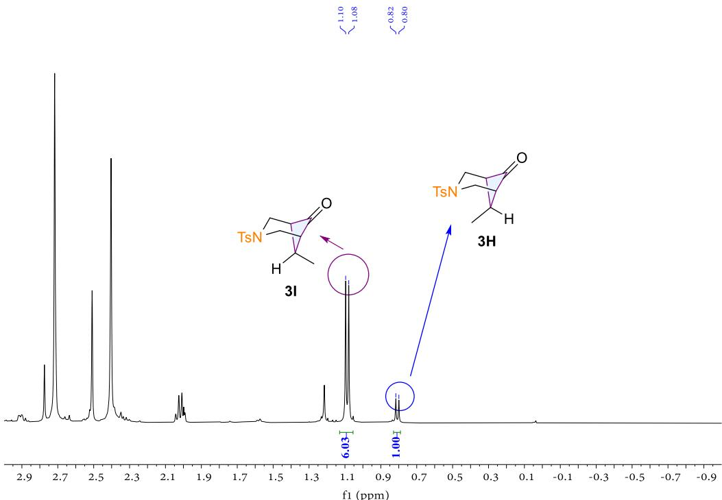
Figure S2. Part of the  $^1\text{H}$  NMR spectrum of the crude products for reaction of **1I'** ( $E/Z = 3:1$ ).
