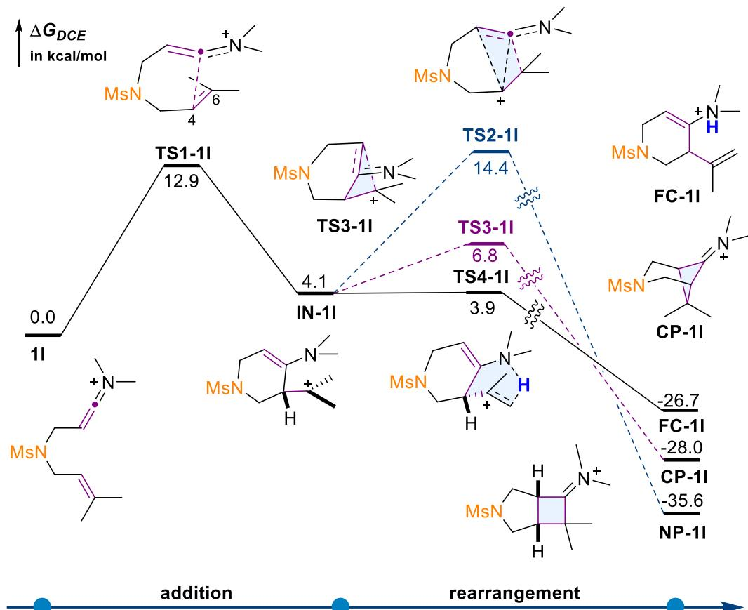
Figure S16. Gibbs energy profile for [2 + 2] cycloaddition and F-C pathway of **1l**. Computed at SMD(DCE)/DLPNO-CCSD(T)/cc-pVTZ// $\omega$ B97X-D/def2-SVP level.
