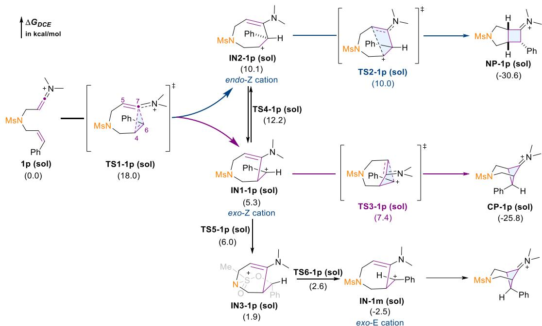
Figure S21. Gibbs energy profile for [2 + 2] cycloaddition of **1p** (structure optimized in solution phase). Computed at DLPNO-CCSD(T)/cc-pVTZ:SMD(DCE)//SMD(DCE)/ $\omega$ B97X-D/def2-SVP level.
