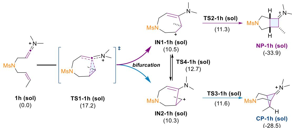
Figure S24. Gibbs energy profile based on solution phase geometry for [2 + 2] cycloaddition of **1h**. Computed at DLPNO-CCSD(T)/cc-pVTZ: SMD(DCE)//SMD(DCE)/ $\omega$ B97X-D/def2-SVP level.
