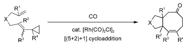
Scheme 1. Rh<sup>I</sup>-catalyzed two-component [(5+2)+1] cycloaddition developed in the Yu group.<sup>[6]</sup>
