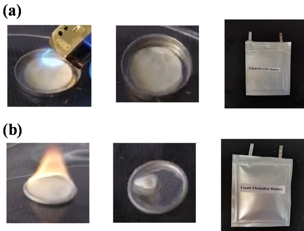
Fig. 2. Comparison between (a) PAEKNW-SPE and (b) commercial PP membrane (Celgard 2325) liquid electrolyte. PAEKNW-SPE doesn't catch fire or deform under open flame. Its soft package battery with Li metal as anode and \text{LiFePO}_4 as cathode doesn't swell after heated under 80^\circ\text{C} for 1 h. On contrast, Celgard 2325 with liquid electrolyte readily catches fire and shrinks significantly, and its battery swells for more than 100% under the same test conditions.
