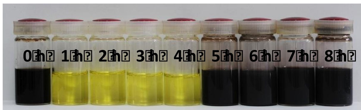
Figure S8. Digital images of the reaction solution for the synthesis of Ru capped column nanocrystals after hydrothermal treatment at 160 °C for different reaction times (0–8 h). The “0 h” sample was the mixture of reagents initially added. Greenish yellow solutions were formed during the first 4 hours of the synthesis, and deep grey to black dispersions were obtained after 5 h of reaction.
