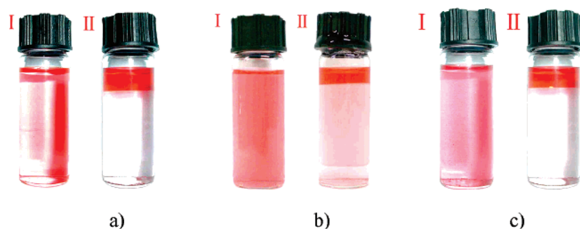
Figure 1. Appearance of mixed solutions with the oil-soluble dye Sudan III (I) below the T_S and (II) above the T_S : (a) 50 mM 1:1.4 DBAB/SL, (b) 50 mM 1.3:1 DEAB/SDSO 3 , and (c) 50 mM 1.3:1 DPAB/SDSO 3 .
