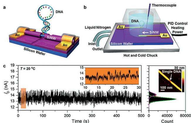
**Figure 1.** a) Diagram of single-hairpin DNA-decorated SiNW biosensors. b) Electrical measurement setup. c) Real-time current recordings of 500 s measured in a PBS solution at  $T = 20^\circ\text{C}$ . Inset shows representative data over a 20 s time interval. The right panel is the corresponding histogram of current values, revealing two Gaussian peaks in conductance. Inset shows an AFM image of a SiNW device, where a single hairpin DNA is attached on the sidewall.
