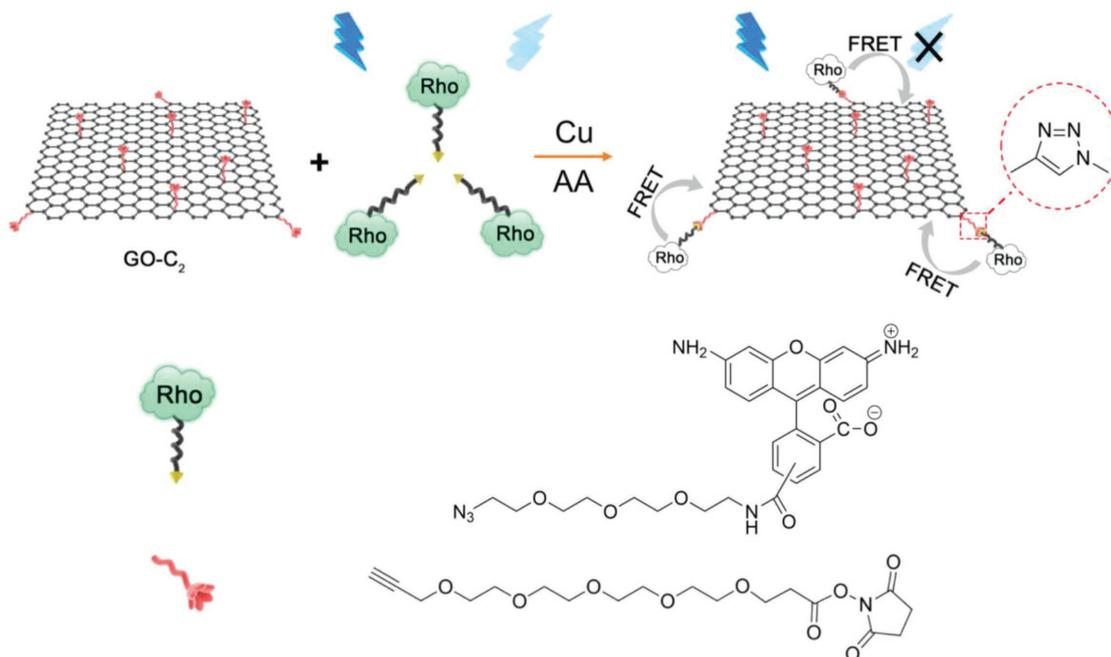
**Figure 1.** Schematic illustration of the Cu detection system based on click chemistry and FRET between GO-C<sub>2</sub> and Rho-N<sub>3</sub>. GO-C<sub>2</sub>: graphene oxide functionalized with alkyne. Rho: carboxyrhodamine110; AA: sodium ascorbate.
