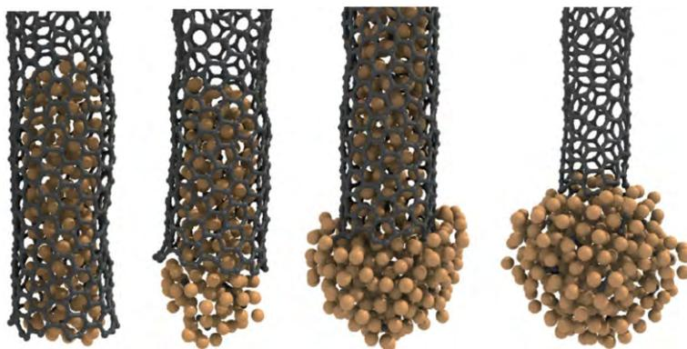
**Fig. 12** Sketch of nanotube/nanoparticle geometries resulting from our Monte Carlo relaxations at 1200 K, ranging from tangential (*left*) to perpendicular (*right*), when C content inside the NP increases. Courtesy Y. Magnin
