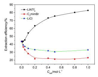
**Fig. 2.** Influence of the concentration of additional salts on the extraction efficiency of Rb<sup>+</sup>,  $C_0$ (Rb<sup>+</sup>) = 23 mmol/L,  $C_{BPC6} = 6$  mmol/L.
