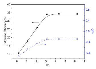
Fig. 3. Extraction efficiency and distribution ratio of  $Rb^+$  at different pH values,  $C_0(Rb^+) = 5.85$  mmol/L.
