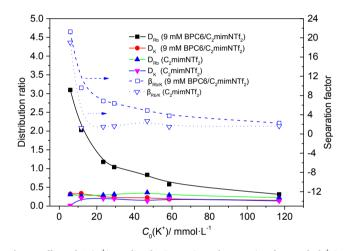
**Fig. 7.** Effect of  $C_0(K^+)$  on distribution ratio and separation factor of Rb<sup>+</sup> in 9 mM BPC6/C<sub>2</sub>mimNTf<sub>2</sub> and pure C<sub>2</sub>mimNTf<sub>2</sub>,  $C_0(Rb^+) = 5.85$  mmol/L.
