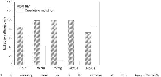
**Fig.** 6. The interference effect of coexisting metal  $C_0(\text{Rb}^+) = C_0(\text{K}^+) = C_0(\text{Na}^+) = C_0(\text{Mg}^{2+}) = C_0(\text{Ca}^{2+}) = C_0(\text{Cs}^+) = 5.85 \text{ mmol/L}.$
