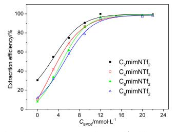
**Fig. 1.** Relationship between extraction efficiency of Rb<sup>+</sup> and the concentration of BPC6 in  $C_n$ mimNTf<sub>2</sub> (n = 2, 4, 6, 8),  $C_0$ (Rb<sup>+</sup>) = 9 mmol/L.
