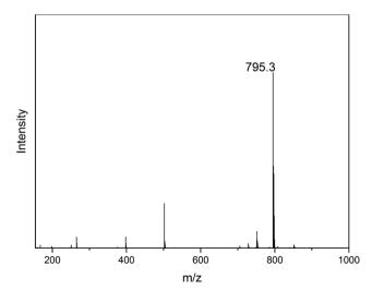
**Fig. 4.** ESI-MS of the IL phase in positive mode after extraction,  $C_0(\text{Rb}^+) = 9 \text{ mmol/L}$ ,  $C_{\text{BPC6}} = 12 \text{ mmol/L}$ .
