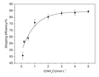
**Fig. 9.** Dependence of Rb<sup>+</sup> stripping efficiency on the NH<sub>4</sub>Cl concentration,  $C_0(\text{Rb}^+) = 5.85 \text{ mmol/L}$ ,  $C_{\text{BPC6}} = 9 \text{ mmol/L}$ .
