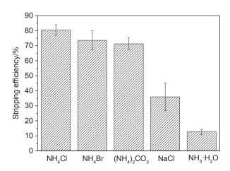
**Fig. 8.** Stripping efficiency by different back extractants,  $C_0(Rb^+) = 5.85 \text{ mmol/L}$ ,  $C_{BPC6} = 9 \text{ mmol/L}$ ,  $C(NH_4Cl) = C(NH_4Br) = C(NaCl) = C(NH_3H_2O) = 2 \text{ mol/L}$ ,  $C((NH_4)_2CO_3) = 1 \text{ mol/L}$ .
