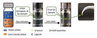
Self-assembly of the uranium-rich SA sample
