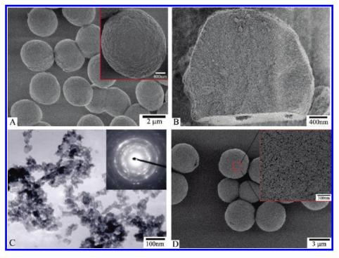
Figure 4. SEM (A, B, D) and TEM (C) images of the samples synthesized at different irradiation times: (A-C) 250 min, (D) 450 min. Insets: (A and D) the image of the corresponding product at higher magnification; (C) the SAED pattern of the corresponding product. The dose rate is 20 Gy/min, and the concentration of EDTA is 8 mmol/L.
