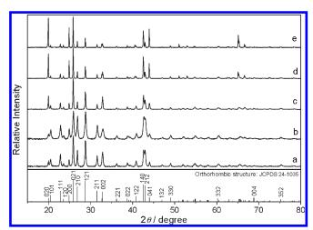
Figure 3. XRD patterns of the samples synthesized under different conditions: (a) irradiation time: 1000 min, [EDTA] = 8 mmol/L; (b) irradiation time: 250 min, [EDTA] = 8 mmol/L; (c) irradiation time:  $1000 \, \text{min}$ ,  $[EDTA] = 0.8 \, \text{mmol/L}$ ; (d) irradiation time:  $1000 \, \text{min}$ , [EDTA] = 0.08 mmol/L; (e) irradiation time: 1000 min, [EDTA] = 0.The dose rate is 20 Gy/min.
