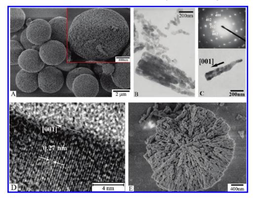
Figure 1. SEM images (A and E), TEM images (B and C), and HRTEM image (D) of the sample synthesized at an irradiation time of 1000 min. The insets in (A) and (C) show the image at higher magnification and the SAED pattern of the corresponding product, respectively. The dose rate is 20 Gy/min, and the concentration of EDTA is 8 mmol/L.
