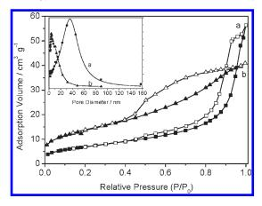
Figure 2. N<sub>2</sub> adsorption (solid)—desorption (open) isotherms of the samples synthesized at different irradiation times: (a) 1000 min, (b) 250 min. The inset shows the pore size distribution of the corresponding samples. The dose rate is 20 Gy/min, and the concentration of EDTA is 8 mmol/L.
