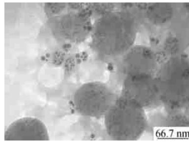
Fig. 4 TEM image of Ag-P4VP hybrid microgels synthesized at the  $\text{Ag}^+$  concentration of 9 mmol/L
