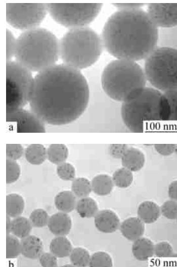
Fig. 6 TEM images of Ag-P4VP hybrid microgels synthesized in the absence (a) and presence (b) of Bis ( $[\text{Bis}] = 2.25 \text{ mmol/L}$ )
