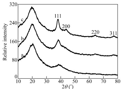
Fig. 3 XRD patterns of Ag-P4VP hybrid microgels synthesized at different dose rate
