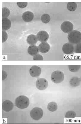
Fig. 2 TEM images of Ag-P4VP hybrid microgels synthesized at the dose rates of 24 Gy/min (a) and 1.7 Gy/min (b)
