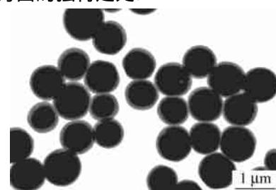
Fig. 7 TEM image of Ag-P4VP hybrid microgels synthesized at the 4-VP concentration of 0.27 mol/L (dose rate: 24 Gy/min)
