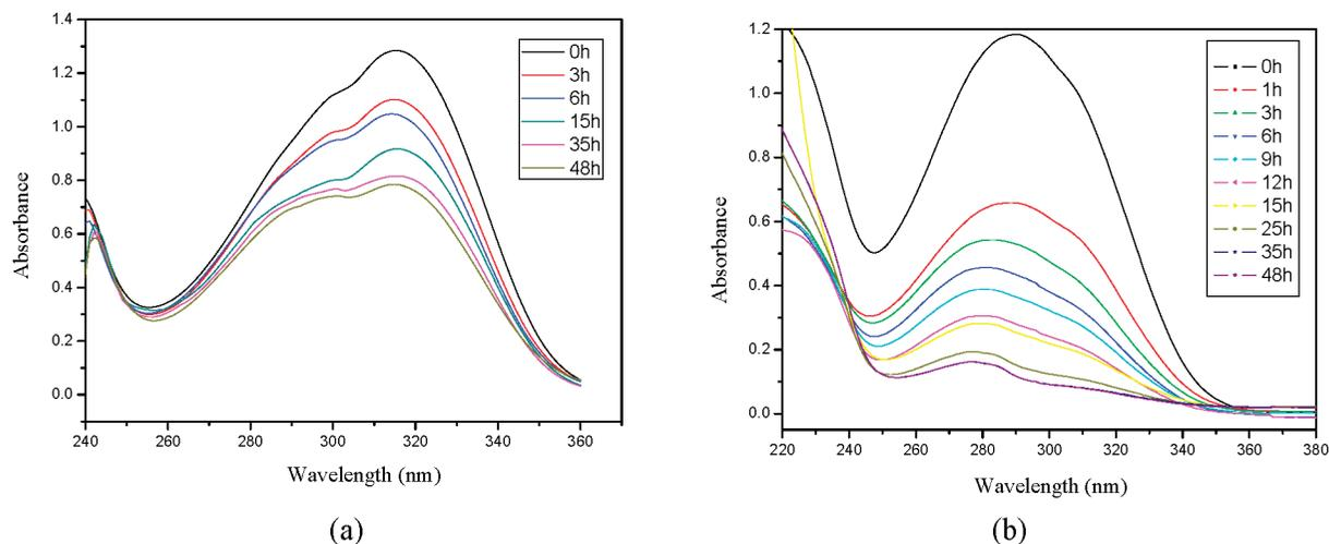
Figure 6. UV/vis spectra change of  $2.5 \times 10^{-5}$  M SDBCC upon irradiation at 30 °C in (a) chloroform and (b) borax buffer.
