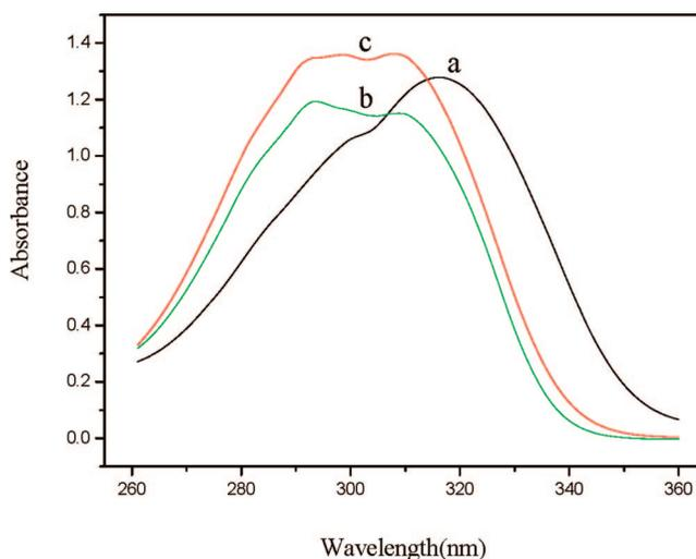
**Figure 4.** UV/vis spectra of  $2.5 \times 10^{-5}$  M SDBCC at 30 °C in (a) methylene dichloride, (b) methanol, and (c) DMSO.
