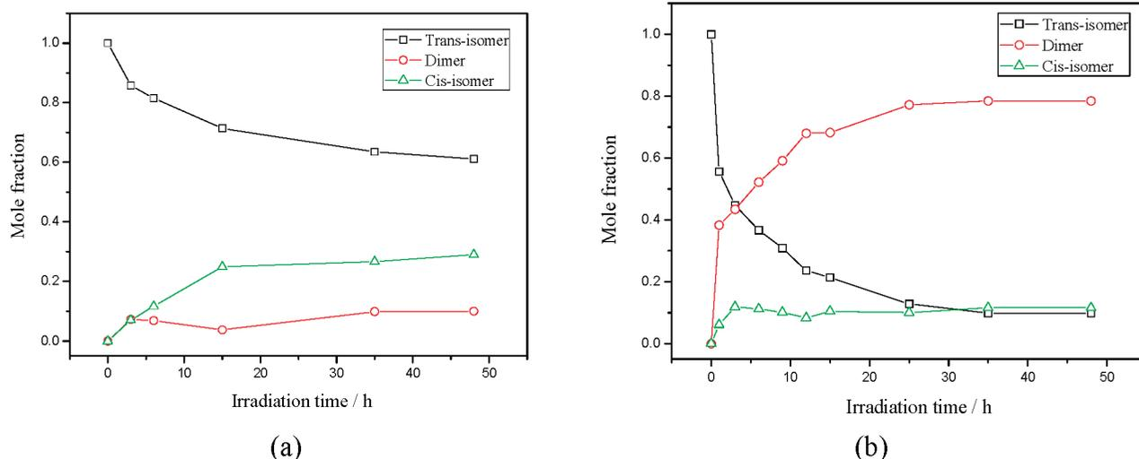
Figure 7. Fractions of trans- and cis-isomers and dimers as a function of irradiation time in (a) chloroform and (b) borax buffer.
