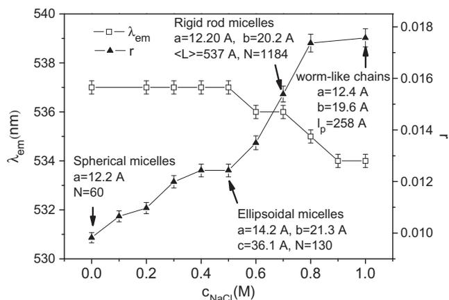
**Fig. 1.** Fluorescence anisotropy and emission maxima of 12-DAN-ADA in SDS/NaBr system ( $C_{\text{SDS}} = 35$  mM,  $C_{12\text{-DAN-ADA}} = 1.0 \times 10^{-6}$  M,  $T = 40$  °C). (The related data of three points in the figure are from the results of SANS and indicating the different micelle type [28]).
