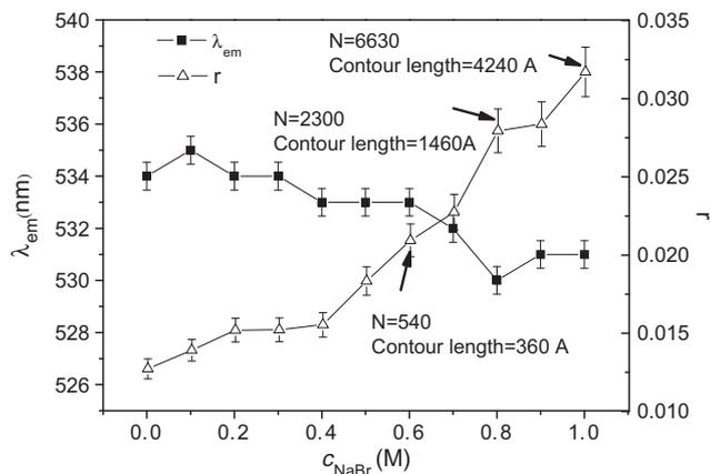
**Fig. 2.** Fluorescence anisotropy and emission maxima of 12-DAN-ADA in SDS/NaBr system ( $C_{\text{SDS}} = 175 \text{ mM}$ ,  $C_{12\text{-DAN-ADA}} = 1.0 \times 10^{-6} \text{ M}$ ,  $T = 40^\circ \text{C}$ ). The related data of three points in the figure are from the results of SANS and indicating the different micelle type [29].
