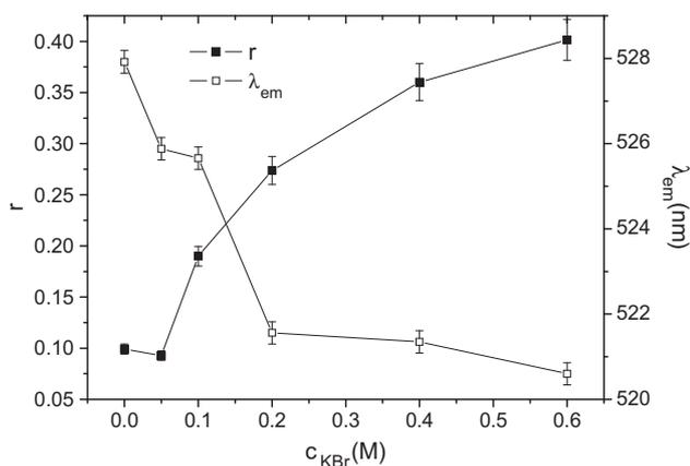
**Fig. 6.** Fluorescence anisotropy and emission maxima of 12-DAN-ADA in CTAB/KBr system in the presence of 0.1 M nitromethane. ( $C_{\text{CTAB}} = 10 \text{ mM}$ ,  $C_{12\text{-DAN-ADA}} = 1.0 \times 10^{-6} \text{ M}$ ,  $T = 30 \text{ }^\circ\text{C}$ ).
