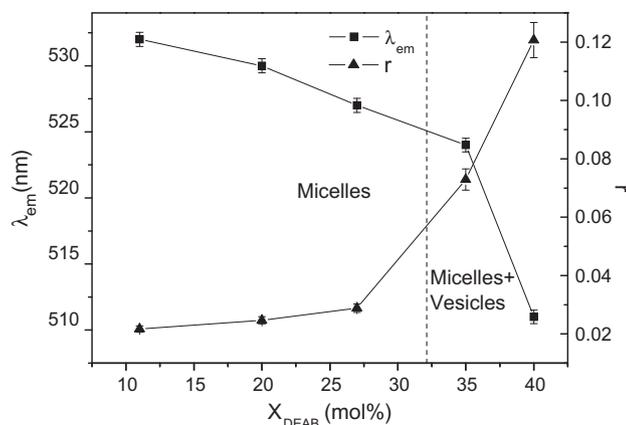
Fig. 7. Fluorescence anisotropy of 12-DAN-ADA in SDS/DEAB system ( $C_T = 200$  mM,  $C_{12\text{-DAN-ADA}} = 1.0 \times 10^{-6}$  M,  $T = 25$  °C).
