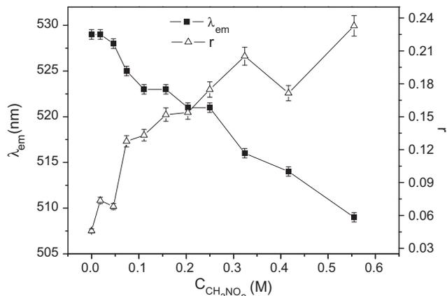
**Fig. 3.** Fluorescence anisotropy and emission maxima of 12-DAN-ADA in different concentrations of nitromethane in 175 M SDS/1 M NaCl system ( $C_{12\text{-DAN-ADA}} = 1.0 \times 10^{-6} \text{ M}$ ,  $T = 40^\circ \text{C}$ ).
