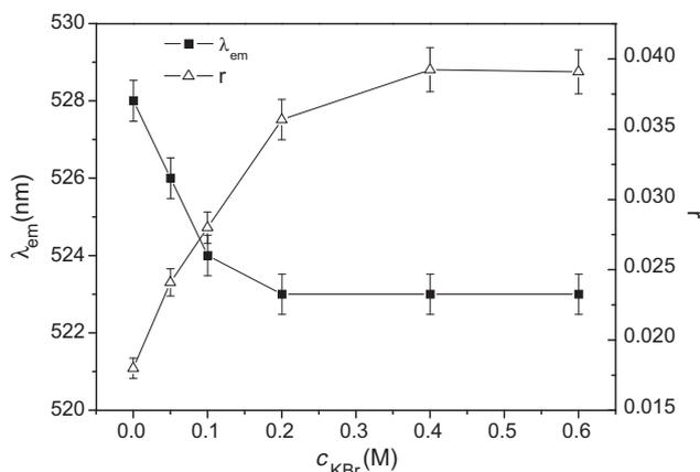
**Fig. 5.** Fluorescence anisotropy and emission maxima of 12-DAN-ADA in CTAB/KBr system ( $C_{\text{CTAB}} = 10 \text{ mM}$ ,  $C_{12\text{-DAN-ADA}} = 1.0 \times 10^{-6} \text{ M}$ ,  $T = 30 \text{ }^\circ\text{C}$ ).
