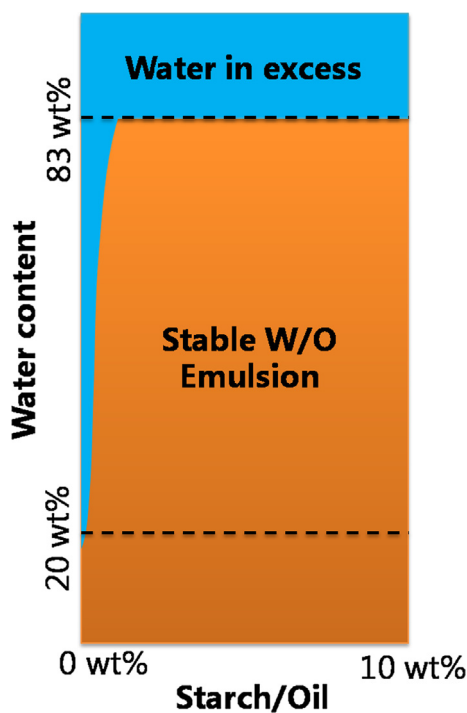
Fig. 2. Phase diagram of emulsions formation. DC8500/SO was 1/1 (w/w) and the dosages of starch 1 were various from 0 wt% to 10 wt% of the DC8500 and SO mixture.
