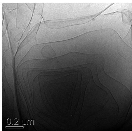
**Fig. 7** Cryo-TEM images of the low viscosity 100 mM CDHEAB at pH 5.78.
