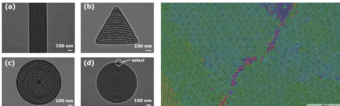
**Left:** Figures a-d, aligned nanowires of platinum, prepared via directed self-assembly. **Right:** large-scale Moiré nanopatterns of ~10 nm silica dots with 3-fold symmetry produced through incommensurate block copolymer self-assembly. Scale bar = 500 nm.
